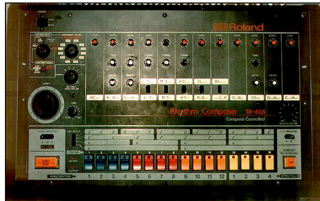
Figure 1: The Roland 808 drum computer: The 16 buttons represent points in time in the step sequencer mode.
